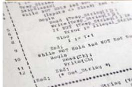
The dot matrix printer printed words in small dots.
